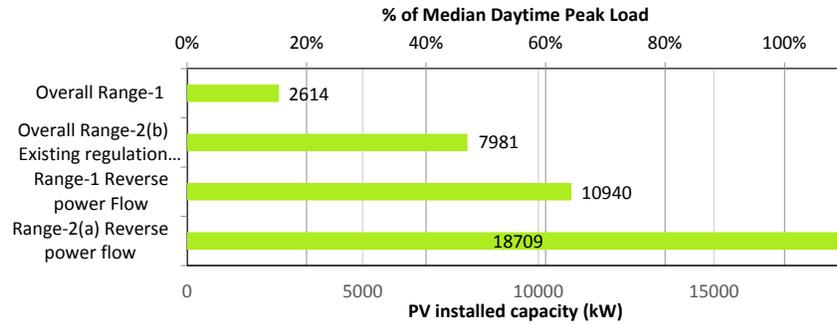
The above analysis to calculate the hosting capacity is performed by a snapshot study considering the worst case when PV is generating at its peak and the load of the circuit is at the representative minimum load value. The tap operations measured in this simulation may not give a correct estimate on total number of tap operations over a day. Therefore, a yearly simulation is performed to calculate the tap operations over the year.
