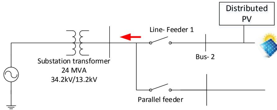
and power factor. However, for this study, the threshold for the reverse power flow is set to be the instant when the power flow reverses at the service transformer and flows towards the substation.
