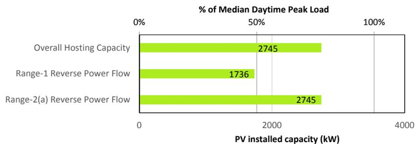
**FIGURE 4-6** Range-2(a) hosting capacity of Circuit B
