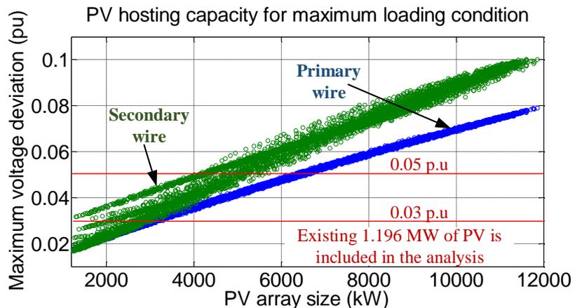
criterion is shown in Figure 3-9. Figures have 10,000 points each, corresponding to 5,000 points of primary (blue pointer) and secondary wires (green pointer), respectively. Every point in Figure 3-8 corresponds to  $V_{max}(x_j^i)$ , i.e. the maximum voltage for the deployment scenario  $x_j^i$ , obtained from load flow analysis.
