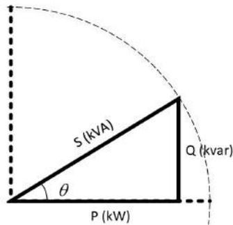
In this smart inverter control mode, the power factor of the inverter is fixed at a particular value. Therefore, reactive power output of the inverter would also be a fixed fraction of the apparent power and it would be according to the relation (5-2).
