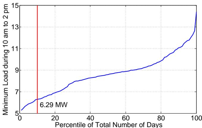
**FIGURE 3-7** Maximum load demand measured at the substation between 10 am to 2 pm.
