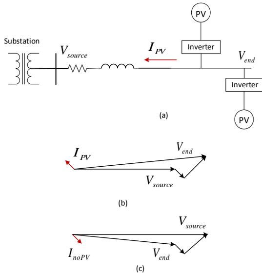
grid, the  $V_{source}$  magnitude is always more than the magnitude at the end of the feeder.
